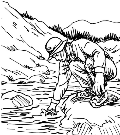
A. Fill plastic water bottle to the brim with river water, leaving zero air in bottle. Cap bottle tightly.
